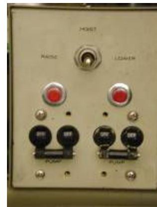
Figure 5 - Bell jar control unit. Use switch on top to control bell jar position.
