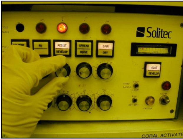
Figure 7 - adjusting the spin rate
