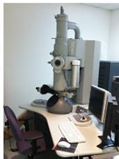
The FEI Tecnai G2 Spirit BT transmission electron microscope is a general-purpose, high resolution instrument that enables the ultrastructural evaluation of biological and non-biological samples with bright-field, dark-field and diffraction modes of operation. The features include:
